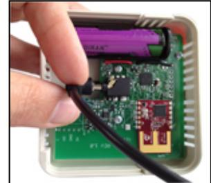
**Controller a second time.** The green PWR/ACT LED located on the front of the Controller will begin to flash at one-second intervals, indicating that the product is operating normally. Power must be 5 volts +/- 10% at 400 milliamp.
